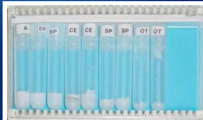
Figure 2. Appearance of a selection of the tubes after three consecutive assays in phase I showing different degrees of standardized synthetic cerumen (SSC) disintegration. As described in Table 1, after test 3, water (A) and Epiotic (EP) did not show any effect on the SSC plug, whereas Cerumene (CE), Specicare (SP) and Otoclean (OT) induced an increasing degree of SSC disintegration and removal.
